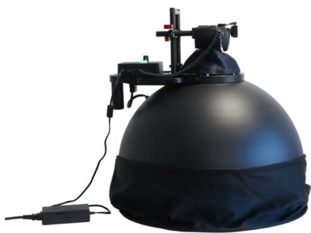
Figure 10: Built-up lighting dome with light protection curtains
