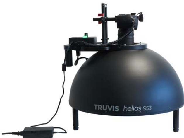
Figure 9: Built-up lighting dome without light protection curtains
